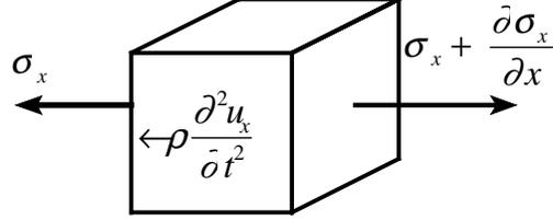
**Figure 16.4. Forces Acting on Unit Cube**
