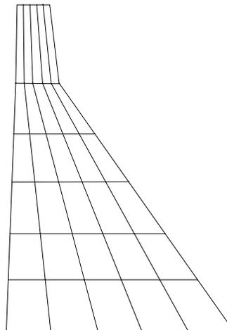
**Figure 16.2.** *Finite Element Model of Dam only*
