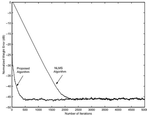
Figure 2: Convergence characteristics of the proposed and NLMS algorithms for the lowest steady-state error reached by the NLMS algorithm,  $\mu_{proposed} = 0.65$ ,  $\mu_{NLMS} = .0055$ .
