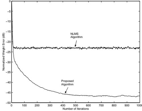
Figure 1: Fastest convergence characteristics of the proposed and NLMS algorithms,  $\mu_{proposed} = 0.55$ ,  $\mu_{NLMS} = 1.00$ .
