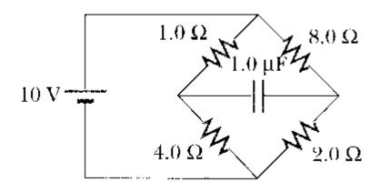
S-28-39 Calculate the power dissipated in each resistor in the figure.
