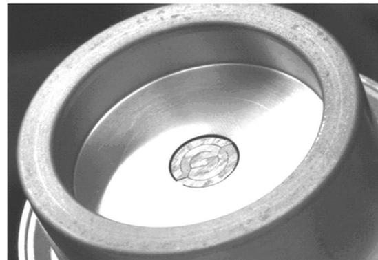
FIG. 11. Details of the Straton cathode. Inside the focusing head, the emitter made of tungsten sheet is visible. The emitter has a diameter of 5 mm.
