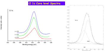
The asymmetry observed in the O 1s spectra is a result of two contributions, one from BO atoms and the other from NBO atoms. From the fitting of the O 1s spectra to two Lorentzian -Gaussian peaks, the ratios BO/O<sub>total</sub> was calculated and found to decrease from 0.426 to 0.188 with an increase in the vanadium content from 0.30 to 0.60.
