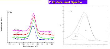
XPS indicates that the BE of the P 2p does not vary much with an increase in V<sub>2</sub>O<sub>5</sub> content. An asymmetry is observed in the P 2p spectra and so fitting of the P 2p was done with two contributions corresponding to P 2p<sub>3/2</sub> and P 2p<sub>1/2</sub>
