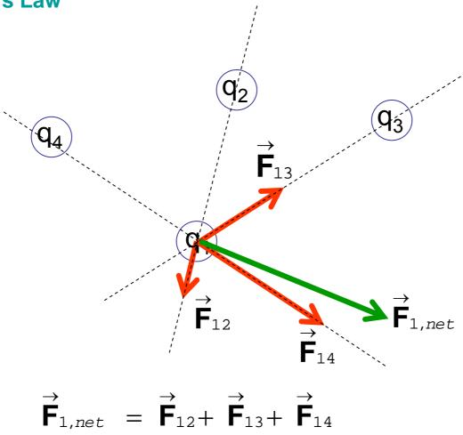
**Principle of superposition**: the net force acting on any particle is the vector sum of the forces acting on this particle due to individual particles
