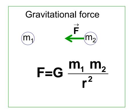
The electrostatic force has the same form as the gravitational force
