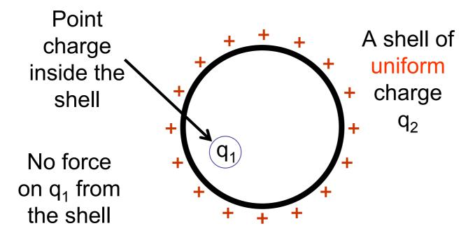
If a charged particle is located inside a shell of uniform charge, there is no net electrostatic force on the particle from the shell.
