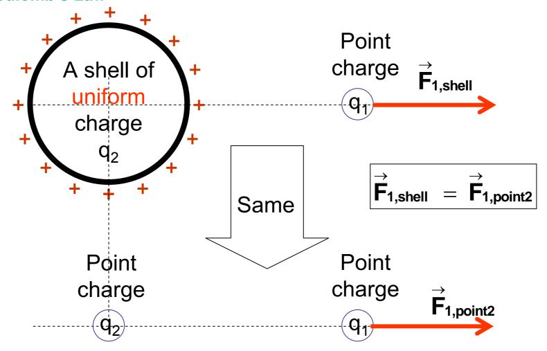
A shell of uniform charge attracts or repels a charged particle that is outside the shell as if all the shell's charge were concentrated at its center
