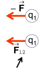
Force on charged particle 1 because of charged particle 2
