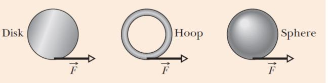
top) by means of strings wrapped around them, with the strings producing the same constant tangential force  $\vec{F}$  on all three objects. The three objects have the same mass and radius, and they are initially stationary. Rank the objects according to (a) their angular momentum about their central axes and (b) their angular speed, greatest first, when the strings have been pulled for a certain time *t*.
