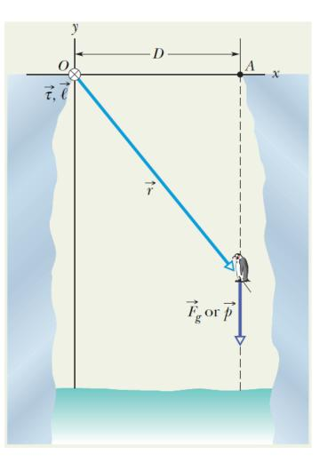
(b) About the origin O, what is the torque  $\vec{\tau}$  on the penguin due to the gravitational force  $\vec{F}_g$ ?
