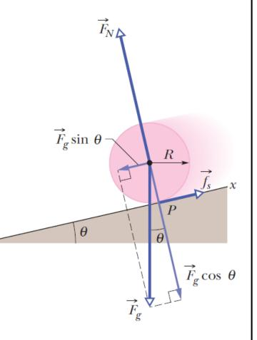
Because the rolling is smooth,  $v_{com} = \omega R$ . The moment of inertial  $I_{com}$  of a sold sphere is  $\frac{2}{5}MR^2$ . Substituting for  $\omega$  and  $I_{com}$  and solving for  $v_{com}$  yield
