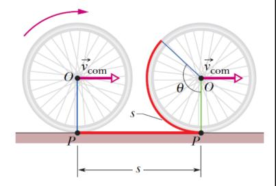
• In the purely rotational motion, every point on the wheel rotates about the center with angular speed  $\omega$ . Every point on the outside edge of the wheel has linear speed  $v_{\rm com}$ .
