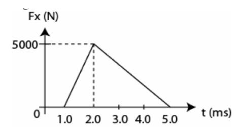
the Im pulse J = area under the curve  $= \frac{1}{2} \times 4.0 \times 10^{-3} \times 5000 = 10 N.s$ but  $J = \Delta p = mv_f - mv_i = m(v_f - v_i) = mv_f$
