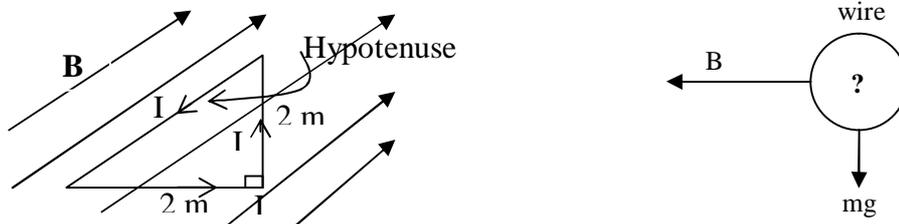
6- A straight horizontal length of copper wire is located in a place where the magnetic field of the earth  $\mathbf{B} = 0.5 \times 10^{-4}$  T (see the figure). What minimum current in the wire is needed to balance the gravitational force on the wire? [The linear density of the wire is 60.0 gram/m] [ $1.2 \times 10^4$  A into the page]
