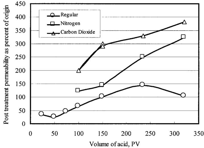
Figure 2. Post-treatment permeability (% of original) vs. PV of acid used.
