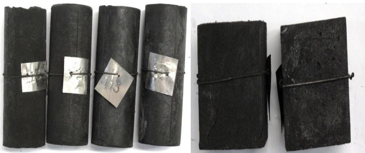
Figure#9: shows some cement samples after being exposed to Formation-A water.
