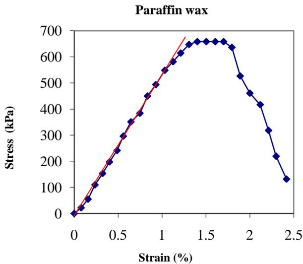
Figure 4. Stress variation with strain for paraffin wax
