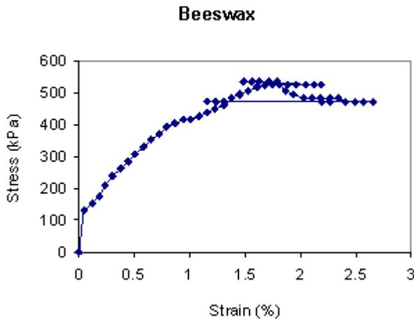
Figure 6. Stress variation with strain for beeswax indicating true load
