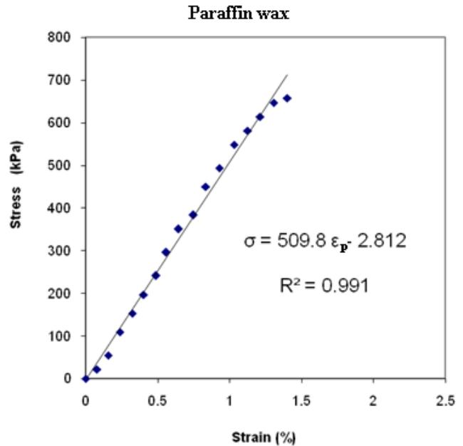
Figure 5. Stress variation with strain for empirical relation based on paraffin wax
