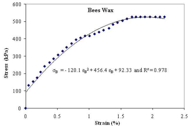
Figure 7. Stress variation with strain for empirical relation based on beeswax
