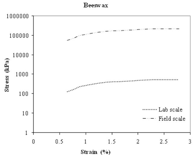
Figure 8. Scaled up stress-strain variation for beeswax in field use
