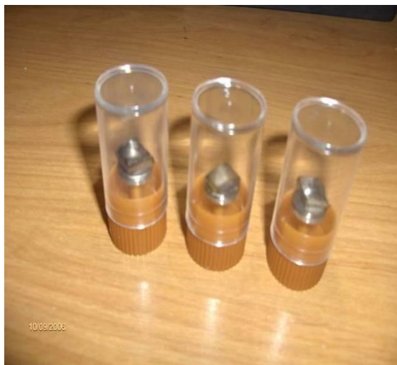
Figure 3. Coated paraffin wax and beeswax samples for SEM tests.
