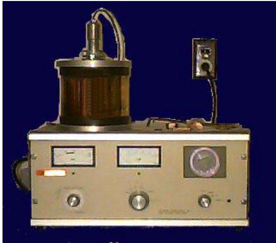
Figure 2. A sputter coater coats the sample with gold-palladium atoms.
