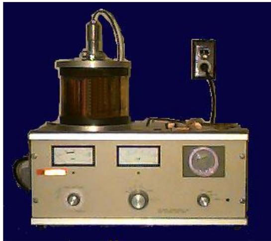
Figure 6. A sputter coater coats the sample with gold-palladium atoms.
