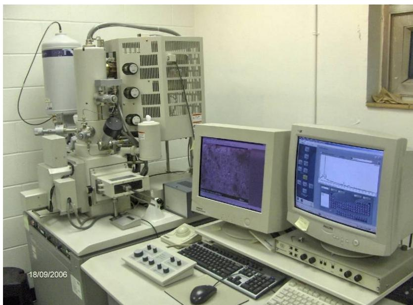
Figure 5. Scanning Electron Microscope (side view)
