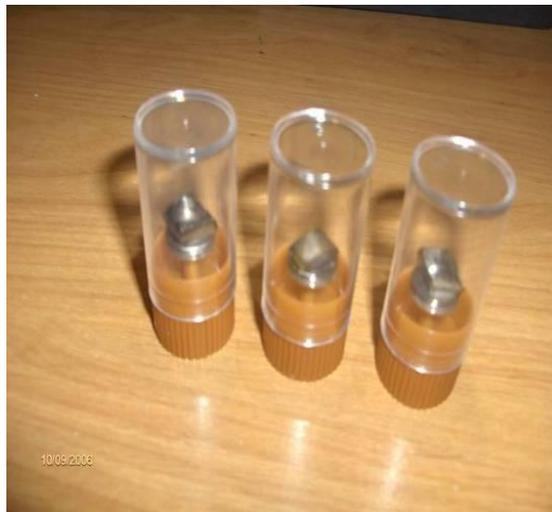
Figure 7. Coated paraffin wax and beeswax samples for SEM tests.
