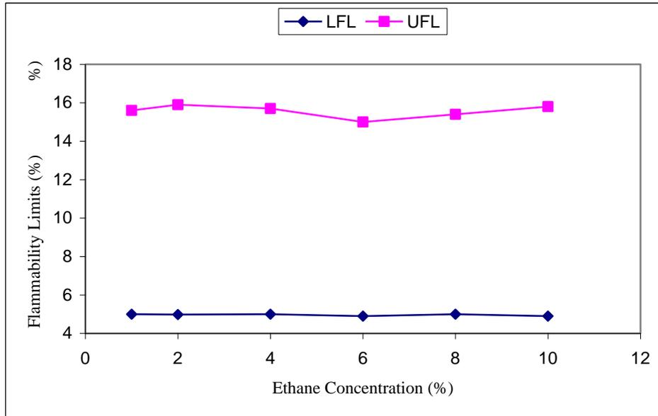
Figure 3. Dependence of NG flammability limits on ethane.
