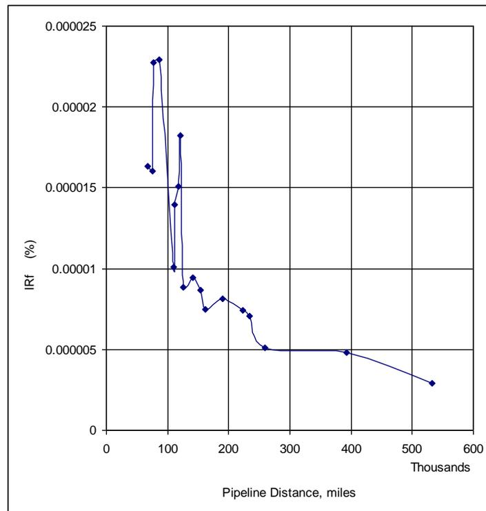
Figure 7. Percent of Individual risk due to flammability with Pipeline Distance.
