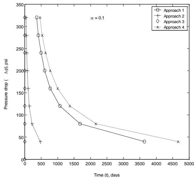
Figure 5. Variation of pressure drop with time for different Approaches.
