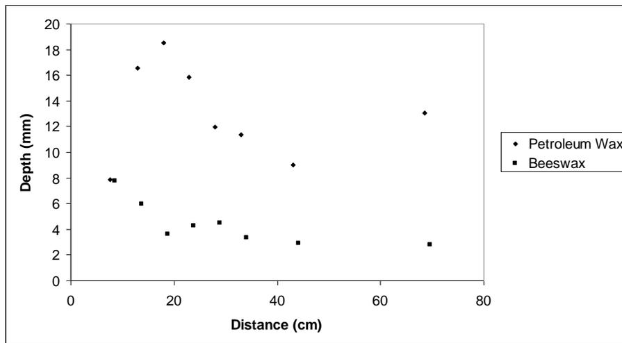
Figure 12. Dependence of DOP on gap distance between drill bit tip and top surface of sample.
