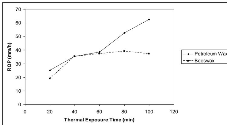
Figure 11. Dependence of ROP on thermal exposure time.
