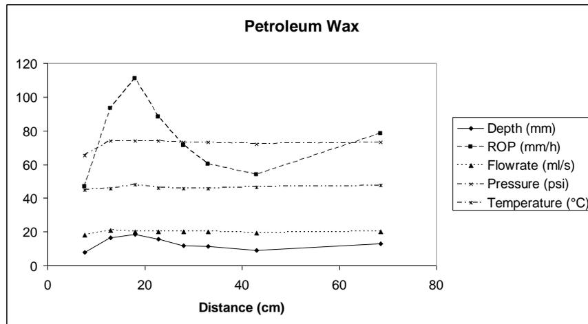
Figure 6. Dependence of different parameters on distance between jet nozzle and paraffin wax sample surface.
