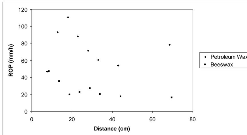
Figure 13. Dependence of ROP on gap distance between drill bit tip and top surface.
