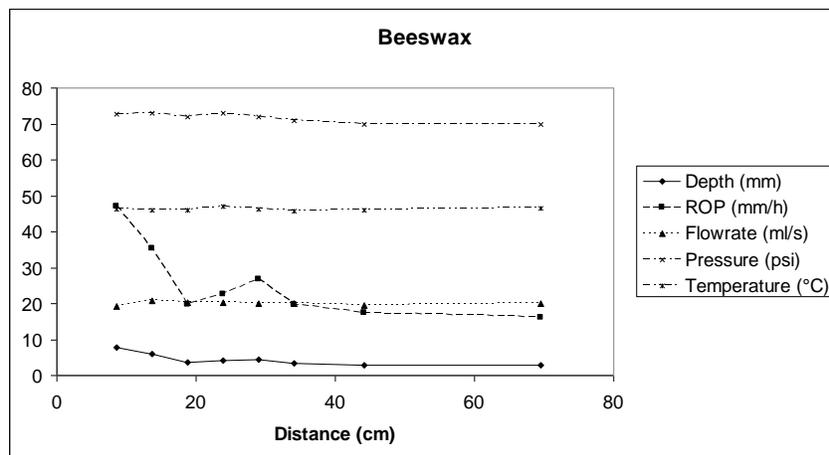
Figure 7. Dependence of different parameters on distance between jet nozzle and beeswax sample surface.
