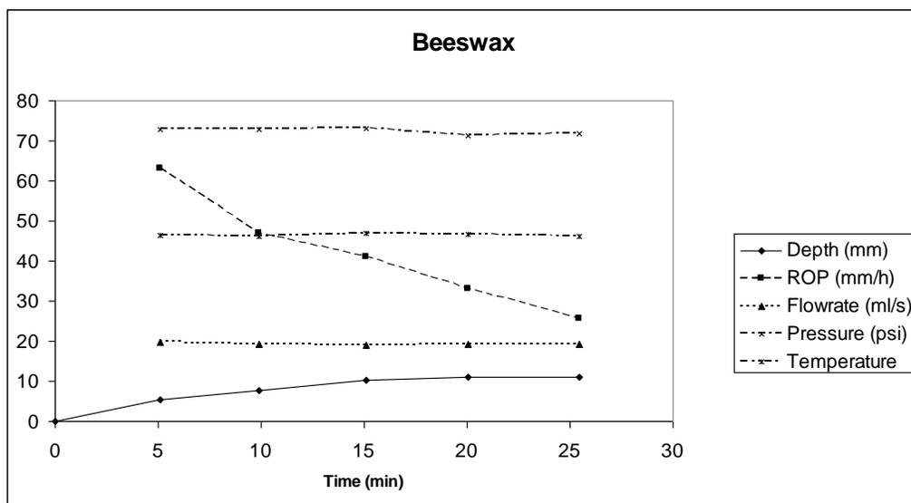
Figure 5. Dependence of different parameters on time for beeswax.
