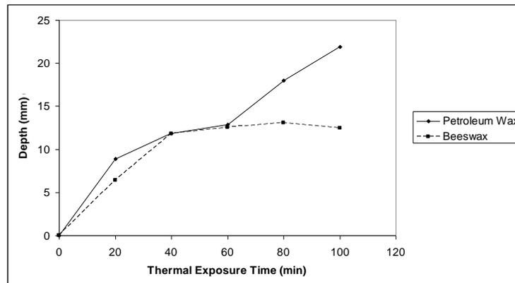
Figure 10. Dependence of DOP on thermal exposure time.
