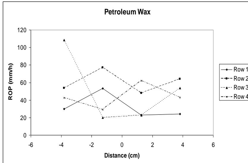
Figure 12. Side effects on rate of penetration (row wise).
