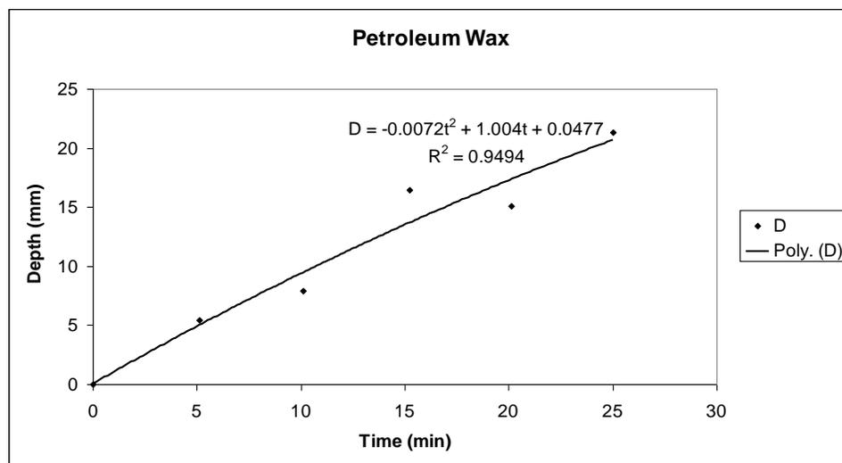
Figure 5. Dependence of depth on time for empirical relation.
