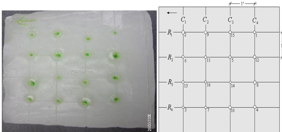
Figure 8. Systematic drilling to investigate side effects.
