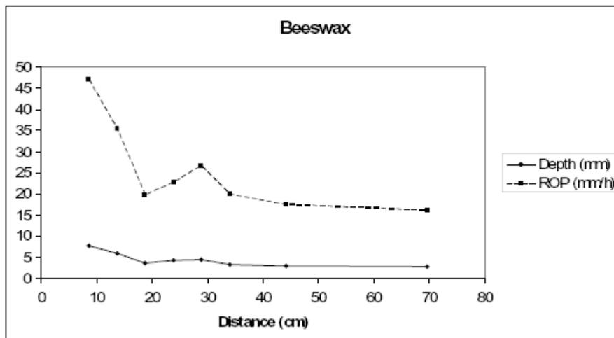
Figure 16. Dependence of depth and ROP on distance between jet nozzle and beeswax surface.
