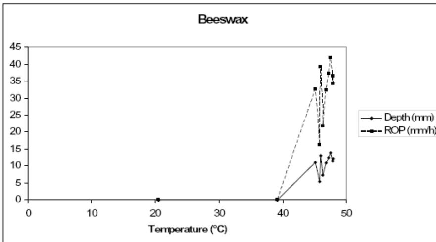
Figure 7. Effects of temperature on depth and rate of penetration.
