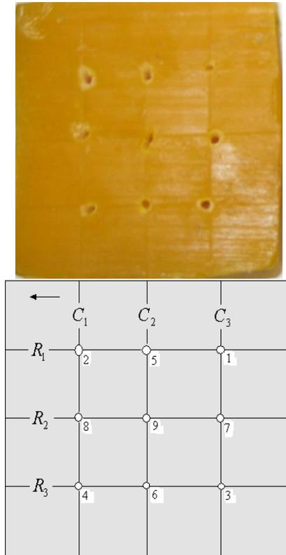
Figure 8. Systematic drilling to investigate side effects.
