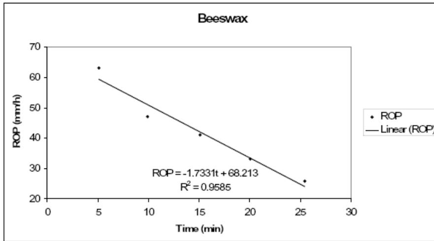
Figure 6. Dependence of rate of penetration on time for empirical relation.
