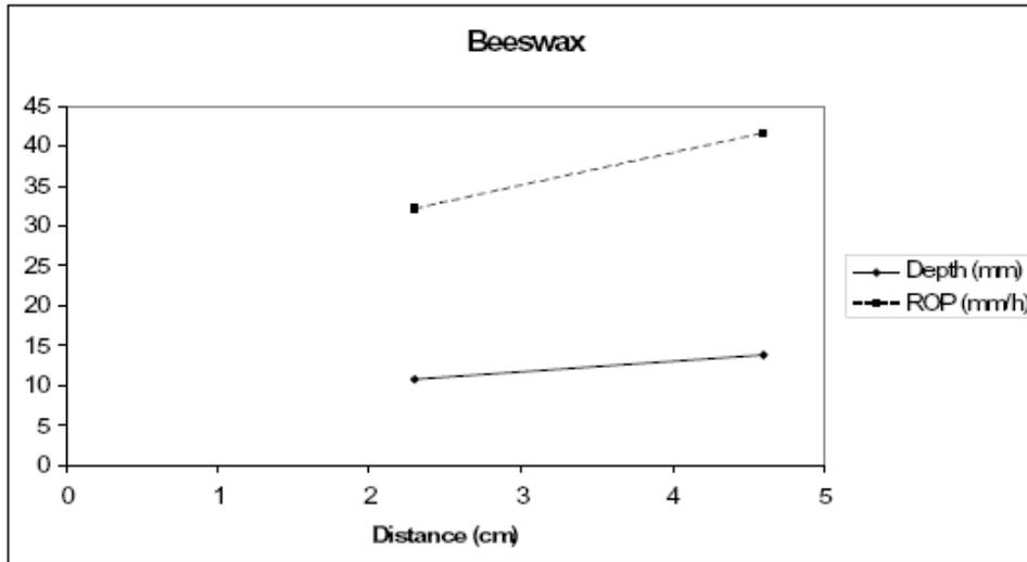
Figure 13. Side effects on depth and rate of penetration (towards centre from edge of the wax sample).
