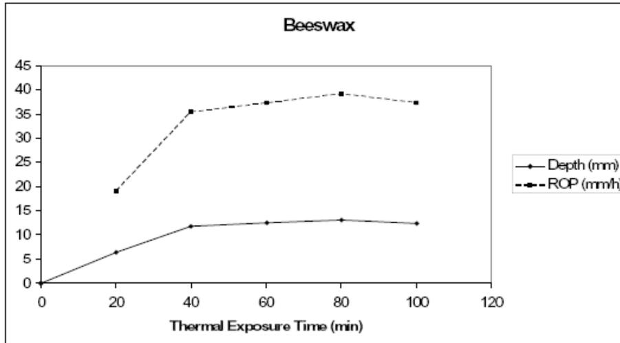
Figure 14. Variation of depth and rate of penetration with thermal exposure time.
