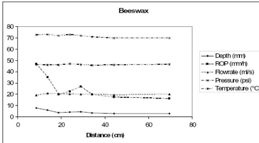
Figure 15. Dependence of different parameters on distance between jet nozzle and beeswax surface.
