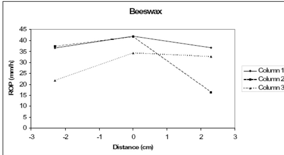
Figure 11. Side effects on rate of penetration (column-wise).
