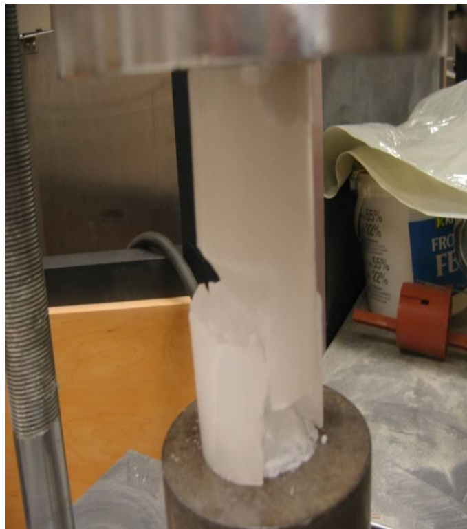
Figure 5. Paraffin wax sample after compressive strength test.
