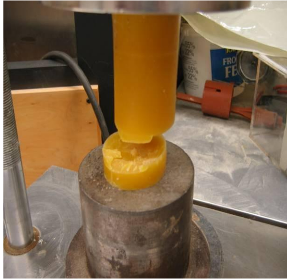
Figure 6. Beeswax sample after compressive strength test.
