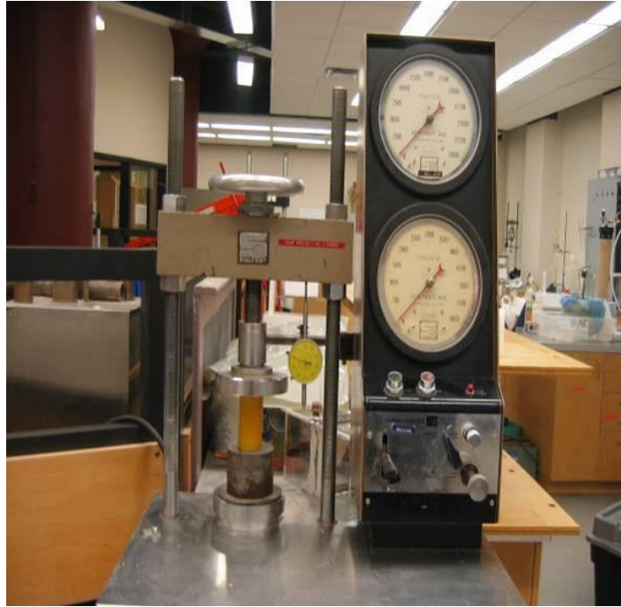
Figure 4. Beeswax sample for compressive strength test.
