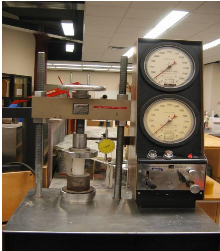
Figure 3. Paraffin wax sample for compressive strength test.
