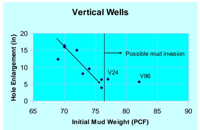
Figure 4. Hole enlargement versus initial mud weight of vertical wells.
