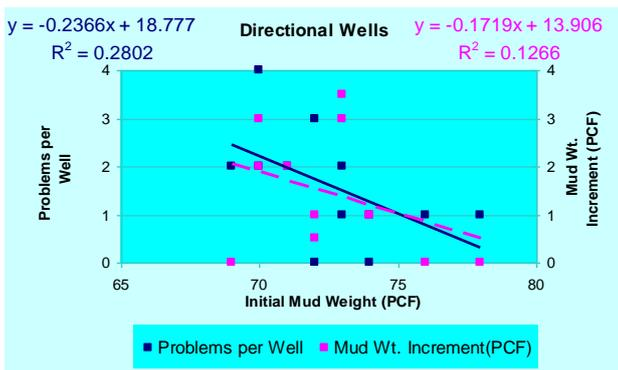
Figure 7. Problems per well and mud weight increment versus initial mud weight of directional wells.
