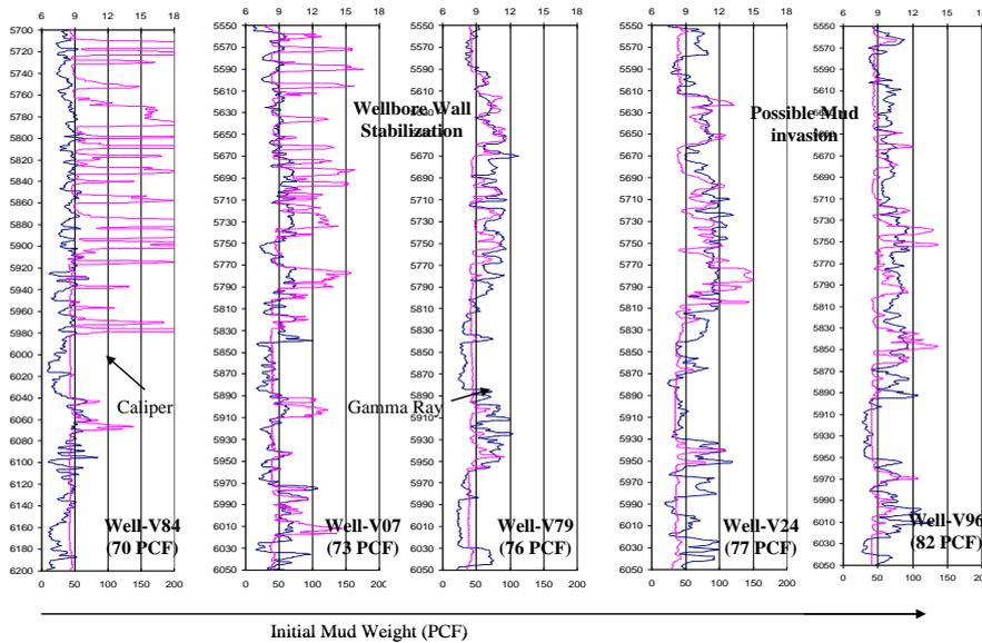
Figure 5. Open hole caliper log of selected vertical wells showing wellbore wall support and possible mud invasion.
