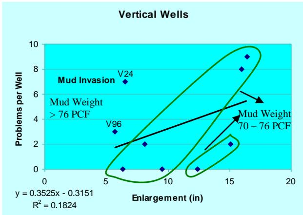
Figure 6. Problems per well versus hole enlargement of vertical wells.
