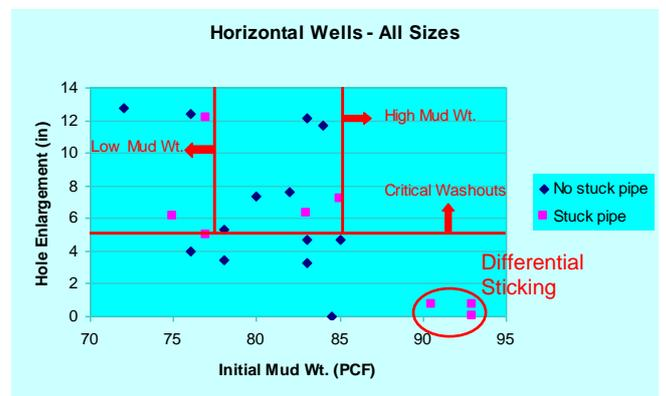
Figure 11. Hole enlargement versus initial mud weight of horizontal wells showing stuck pipes – definition of critical washouts.
