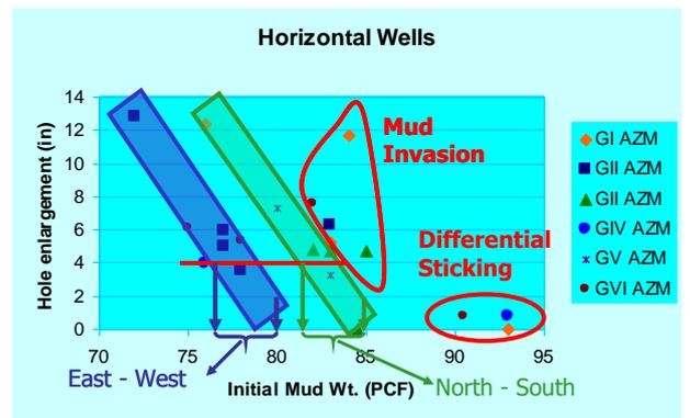
Figure 10. Hole enlargement versus initial mud weight of horizontal wells – identification of mechanisms and design of safe mud weight window.
