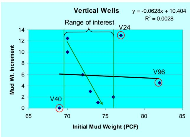
Figure 2. Mud weight increment versus initial mud weight of vertical wells.
