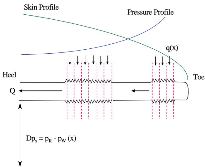
**Fig.A-1, Horizontal Well Schematic Diagram, Showing Expected Skin and Pressure Profiles.**
