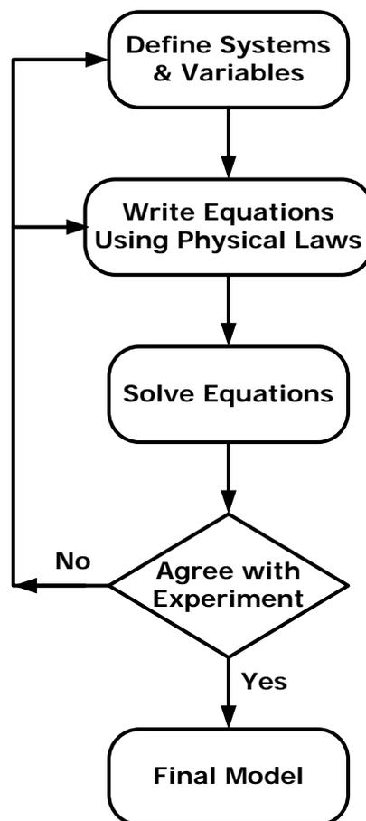
Figure 1-4 Flowchart for the mathematical modeling procedure
