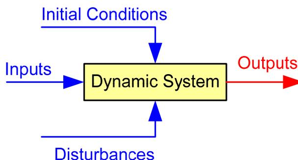
Figure 1-1 Excitation and response of a system
