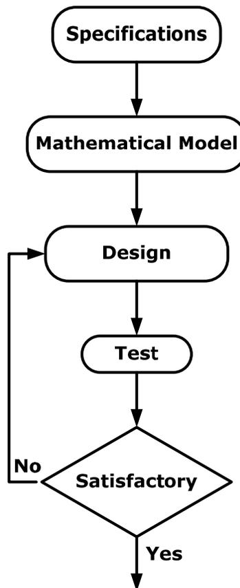
Figure 1-5 Flowchart for the analysis and design of dynamic systems
