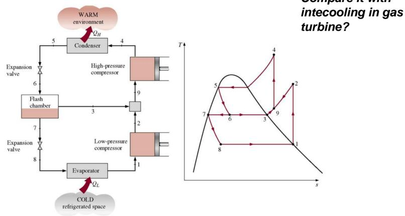
Instead of throttling from 5 to 8' directly, we make two stage throttling (similar to two stage turbines !). We throttle from 5 to 6, use the low temp vapor to cool the compressed vapor from 2 to 9.
