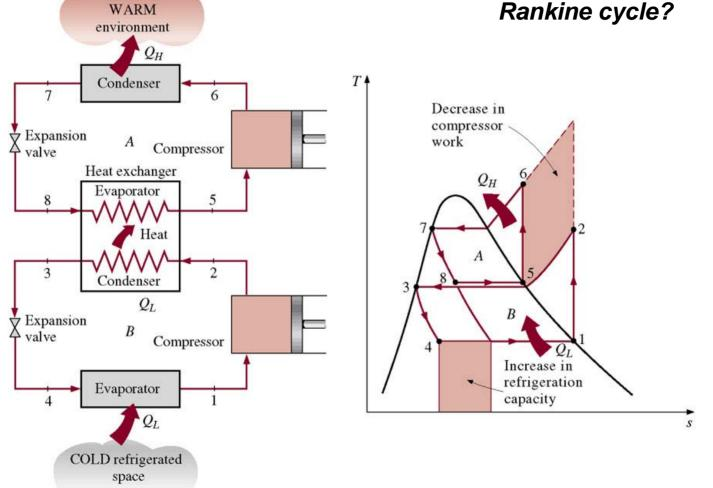
A two-stage cascade refrigeration system with the same refrigerant in both stages. SOLVE EXAMPLE 10-3
