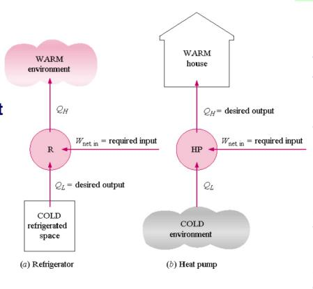
The objective of a *heat pump* is to maintain a heated space at a high temperature. This is accomplished by absorbing heat from a low-temperature source, such as well water or cold outside air in winter, and supplying this heat to a warmer medium such as a house,
