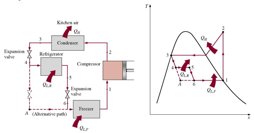
We throttle first from 3 to 4, absorb heat from the refrigerator, then throttle again from 5 to 6 and absorb heat from the freezer.
