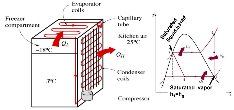
State 2: P2 and s2 => superheated vapor =>interpolate and get h2 State 4: h4=h3 (throttling process)
