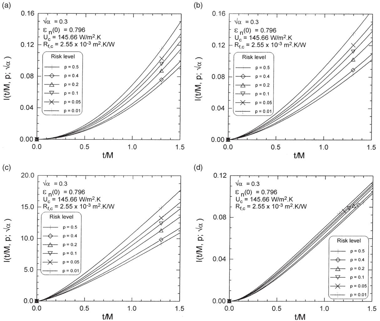
Fig. 6. The representation of the effectiveness degradation function  $I(t,p;\sqrt{\alpha})$  as a function of reduced time  $t/M$  with different values of risk level  $p$  and scatter parameter  $\sqrt{\alpha}=0.30$  (a) linear; (b) power-law with exponent  $n=0.50$  ; (c) falling rate; and (d) exponential fouling growth models.
