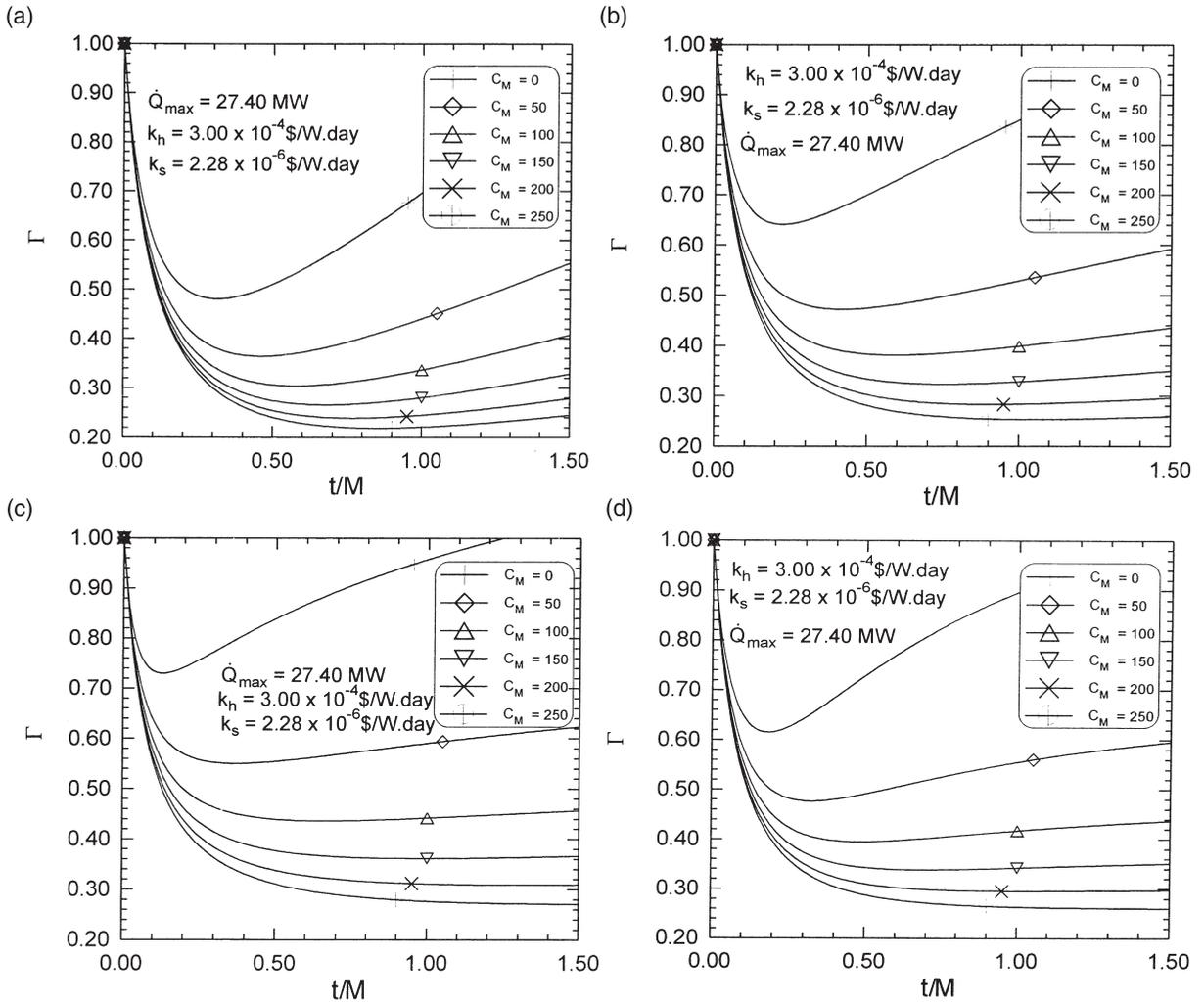
Fig. 4. The effect of miscellaneous cost  $C_M$  on the total dimensionless cost for a deterministic case  $p=0.50$  (a) linear; (b) power-law with exponent  $n=0.50$  ; (c) falling rate; and (d) exponential fouling growth models.
