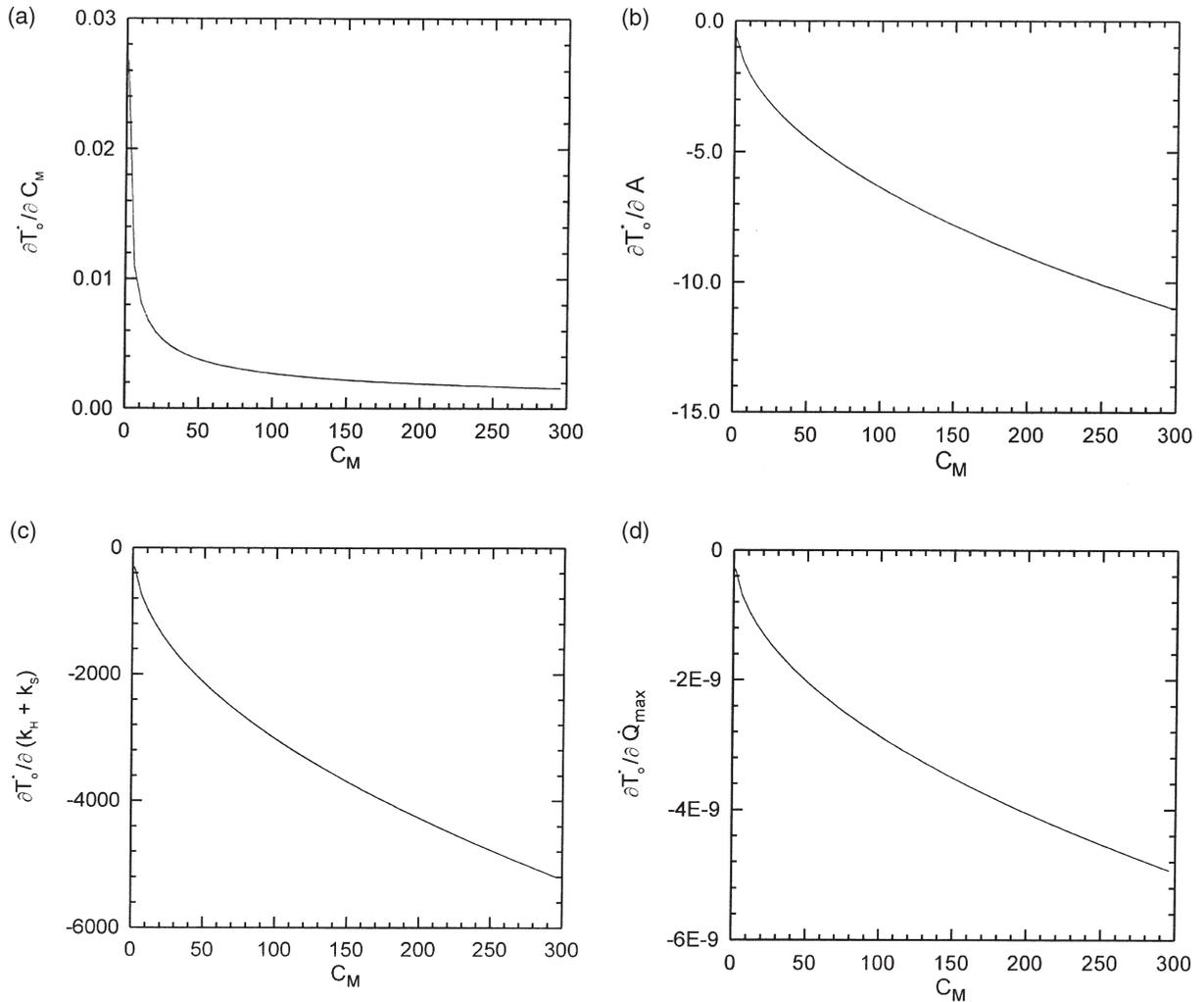
Fig. 8. The sensitivity of dimensionless cycle time  $T_0 \approx t$  with respect to different thermal-cost parameters  $C_M$ ,  $A$ ,  $(k_H + k_S)$  and  $Q_{\max}$  as function of miscellaneous cost  $C_M$  for a linear model: the parameters are same as those given in Table 1.
