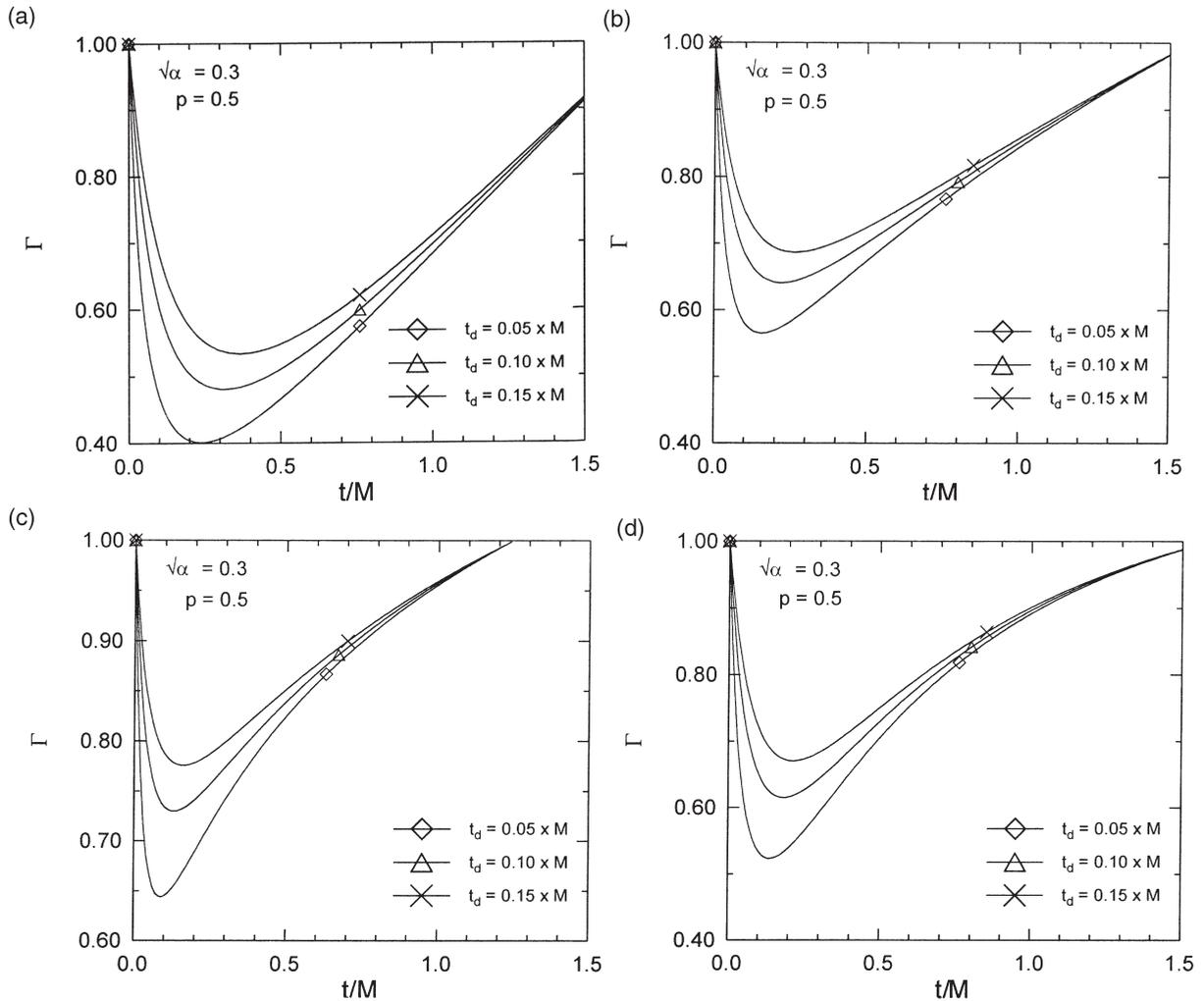
Fig. 3. The effect of down time  $t_{down}$  on the total dimensionless cost for a deterministic case  $p=0.50$  (a) linear; (b) power-law with exponent  $n=0.50$ ; (c) falling rate; and (d) exponential fouling growth models.
