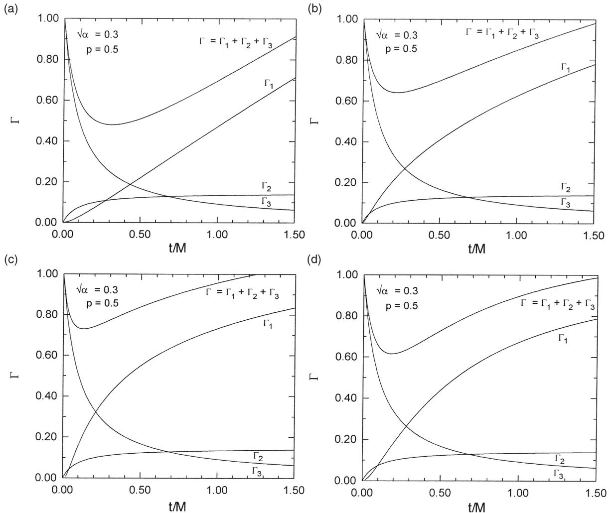
Fig. 5. The effect of various cost elements ( $\Gamma_1, \Gamma_2, \Gamma_3$ ) to the total dimensionless cost ( $\Gamma = \Gamma_1 + \Gamma_2 + \Gamma_3$ ) for a deterministic case  $p = 0.50$  (a) linear; (b) power-law with exponent  $n = 0.50$ ; (c) falling rate; and (d) exponential fouling growth models.
