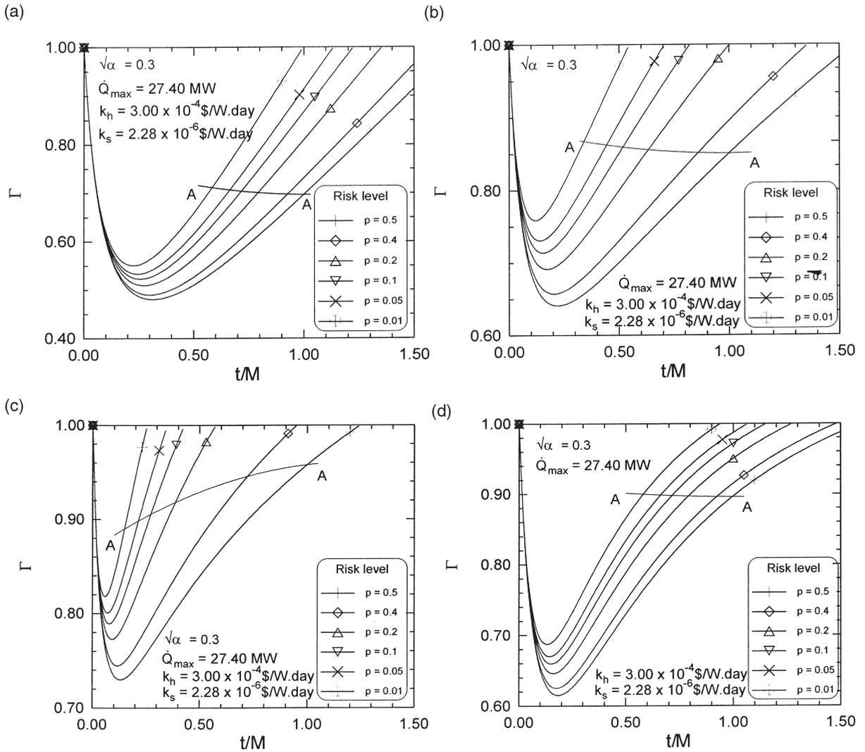
Fig. 2. Dimensionless total cost vs dimensionless operating time with different values of risk level  $p$  and scatter parameter  $\sqrt{\alpha}=0.30$  (a) linear; (b) power-law with exponent  $n=0.50$ ; (c) falling rate; and (d) exponential fouling growth models.
