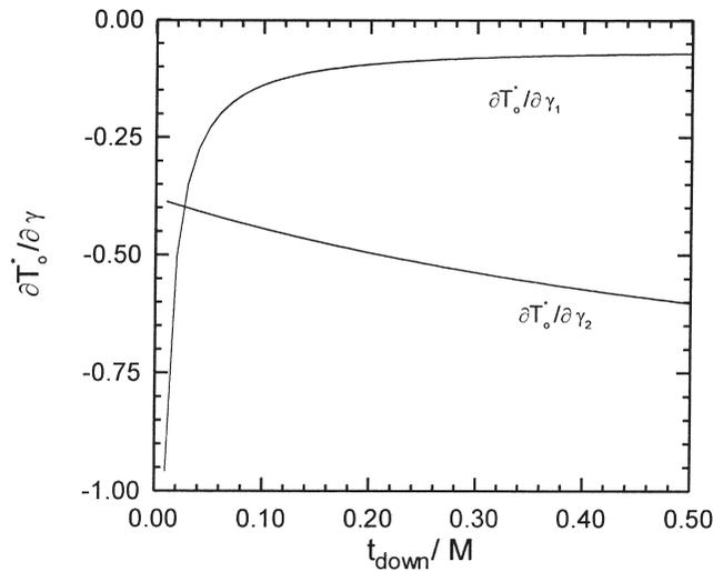
Fig. 7. The sensitivity of dimensionless cycle time  $T_0=t+t_{\text{down}}$  with respect to the cost parameters  $\gamma_1$  and  $\gamma_2$  as function of reduced downtime  $t_{\text{down}}/M$  for a linear model; the parameters are same as those given in Table 1.
