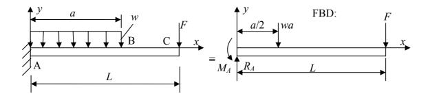
First we draw a FBD for the system to find the reactions, which are found from Newton's equations as  $R_A = F + wa$  and  $M_A = FL + wa^2/2$ . We then cut the beam between A-B and B-C to find the bending moments of  $M_{AB}$  and  $M_{BC}$  as:
