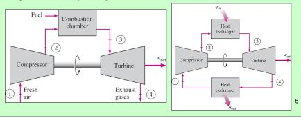
The ideal cycle that the working fluid undergoes in this closed loop is the **Brayton cycle**, which is made up of four internally reversible processes:
