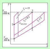
For fixed values of  $T_{\rm min}$  and  $T_{\rm max}$ , the net work of the Brayton cycle first increases with the pressure ratio, then reaches a maximum at  $W_{net,max}$  and finally decreases.
