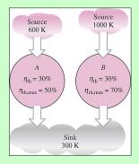
$$\begin{split} &\eta_{rev,A} = \left(1 - \frac{T_L}{T_H}\right)_A = 1 - \frac{300}{600} = 50\% \\ &\eta_{rev,B} = \left(1 - \frac{T_L}{T_H}\right)_B = 1 - \frac{300}{1000} = 70\% \end{split}$$
