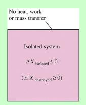
$$\Delta X_{\text{isolated}} = (X_2 - X_1)_{\text{isolated}} \le 0$$
