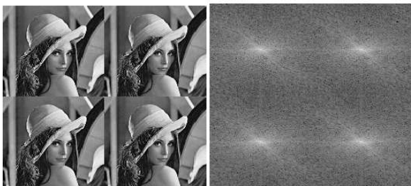
Fig. 3. Balanced multiwavelet approximation subband of Lena image (left). Spectral densities of subband blocks L_0L_0 , L_0L_1 , L_1L_0 and L_1L_1 (right).
