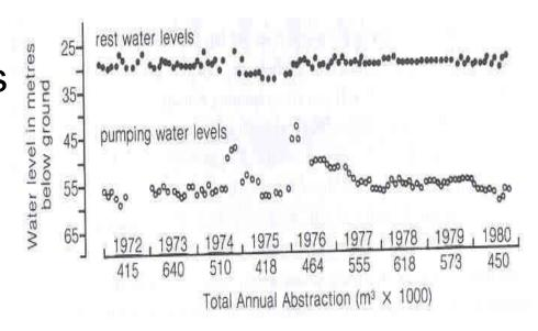
Reflects the affect of pumping on groundwater aquifers (groundwater decline due to increased pumping)
