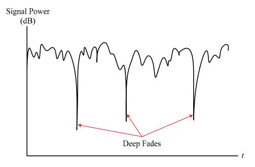
During the time instants where fading is so sever (during deep fades) data that is transmitted may be lost and impossible to recover back. To avoid losing data due to deep fades as much as possible the concept of diversity combining is employed.
