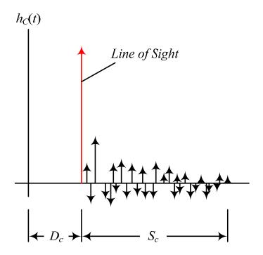
where  $D_c$  is the channel delay that represents the time the first electromagnetic component takes to travel from the transmitter to the receiver, and  $S_c$  is the spread of the channel representing the time
