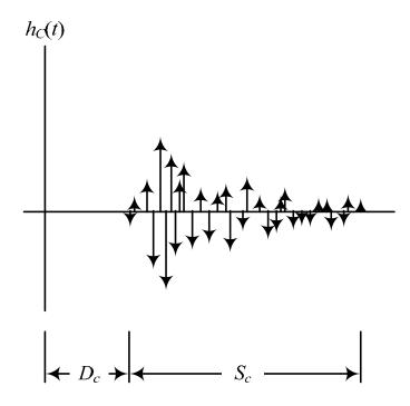
The effect of the spread of the channel is the smearing (spreading) of the transmitted signal at the receiver. This effectively causes the transmitted bits of a digital signal to get mixed together (intersymbol interference)
