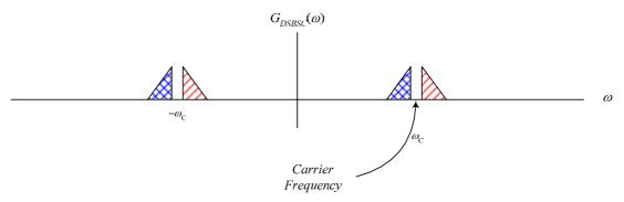
Clearly, in this case, the use of a narrowband BPF to extract the carrier frequency from the modulated signal is not possible because no components in the modulated signal fall at the carrier frequency. Therefore, another method must be used in general.
