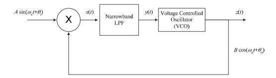
Voltage-Controlled Oscillator (VCO): is a device that produces a sine wave with a frequency that is linearly proportional to the value of the input signal (when the input increases, the frequency of the output increases and vice versa). The frequency of the output of the VCO when the input is zero is called the Free Running Frequency (FRF).
