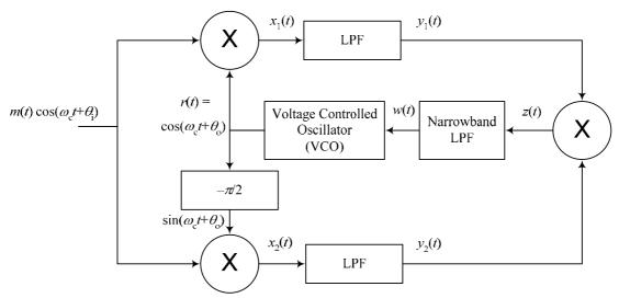
The signals  $x_1(t)$  and  $x_1(t)$  in the block diagram above are simply obtained by multiplying the received DSBSC modulated signal respectively by  $\cos(\omega_c t + \theta_o)$  and  $\sin(\omega_c t + \theta_o)$ , which is obtained by shifting  $\cos(\omega_c t + \theta_o)$  by  $-\pi/2$ . So,
