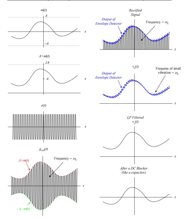
The following figure illustrates modulation and demodulation of AM in frequency—domain (Note: the demodulation techniques used above and below are slightly different (above an envelope detector is used and below, a rectifier detector is used)).
