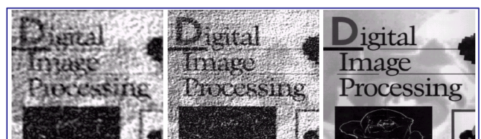
FIGURE 5.30 Results of constrained least squares filtering. Compare (a), (b), and (c) with the Wiener filtering results in Figs 5.29(c), (f), and (i), respectively.
