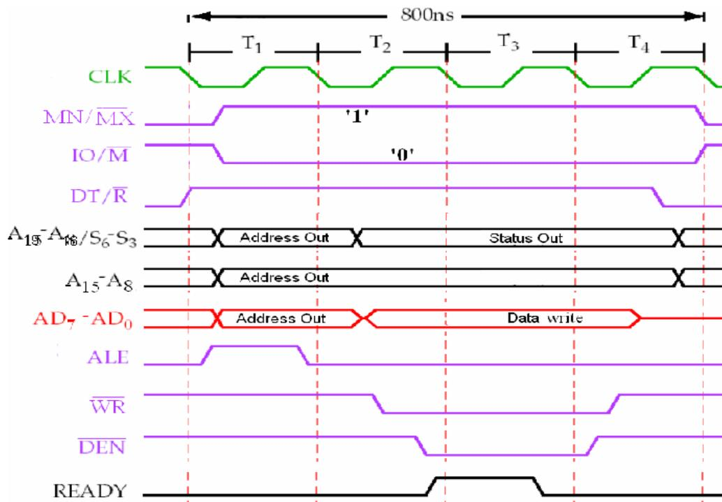
**Note:** Note that the control signal logic levels and timing diagram are similar to that of read operation, except for data transmit or receive mode, read and write signals.
