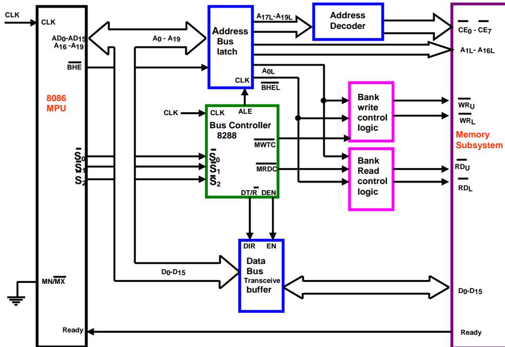
**Note:** The Bus controller is introduced here due to the support of multiprocessor environment of Maximum mode. The decoder is used to select desired memory chips. The remaining components of this circuit are similar to 8088 minimum mode circuit, as shown in [slide 1](#).
