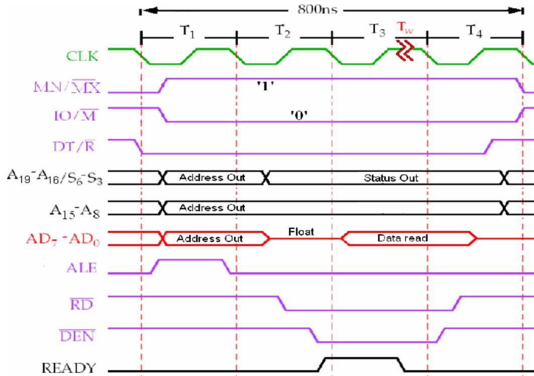
**Note:** Note that during T<sub>1</sub> or the 1<sup>st</sup> clock pulse, the read bus cycle starts and valid address is latched together with setting minimum and maximum mode, input output or memory interface, data transmit and receive mode of buffer IC.
