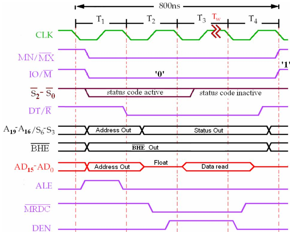
**Note:** Note that in maximum mode status codes needs to be active to generate control signals from bus controller.
