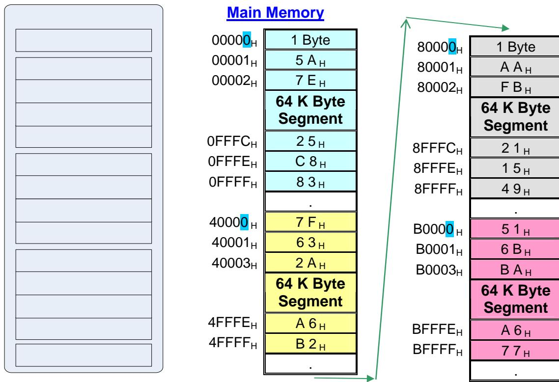
**Solution:** This instruction involves the Code-segment and will only affect the CS and IP registers of the CPU. Since the Base address of the Code-segment is specified to be  $B000_{\text{H}}$ , the segment-address (SA) part of the PA that will be loaded into the CS register will be ' $B000_{\text{H}}$ ', and the offset-address (OA) part of the PA that will be loaded into the IP register will be ' $1234_{\text{H}}$ '.
