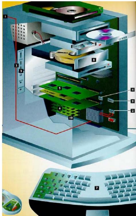
**1** The CPU uses the address to find and invoke the ROM BIOS boot program, which in turn invokes a series of system checks. The CPU first checks itself and the POST program by reading code loaded into various locations and checking it against identical records stored permanently in the BIOS chip set.
