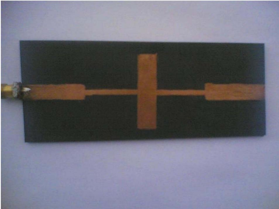
This filter is examined by the Network Analyzer and the response is the following:
