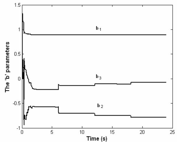
**Figure 7** Online adaptation of the 'b' parameters
