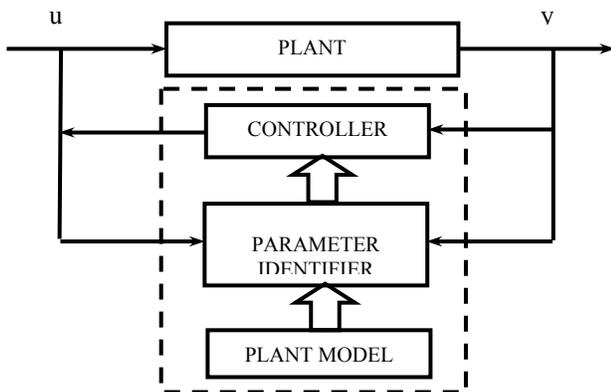
Figure 2 Block diagram of self-tuning controller
