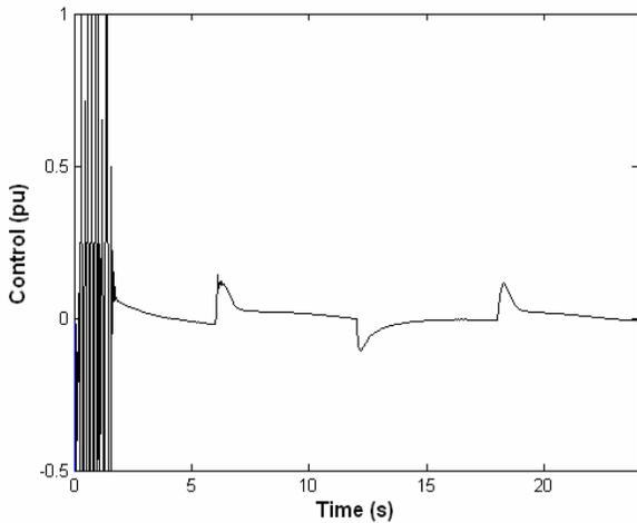
**Figure 8** The control signal using the pole-shift method
