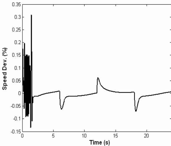
**Figure 4** Generator speed deviation with the online adaptive stabilizing control
