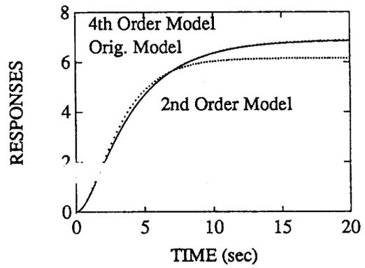
Figure 4. Step response  $y_2$  to input  $u_2$
