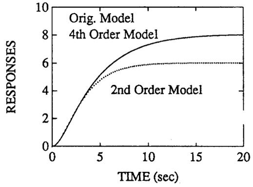
Figure 2. Step response  $y_2$  to input  $u_1$
