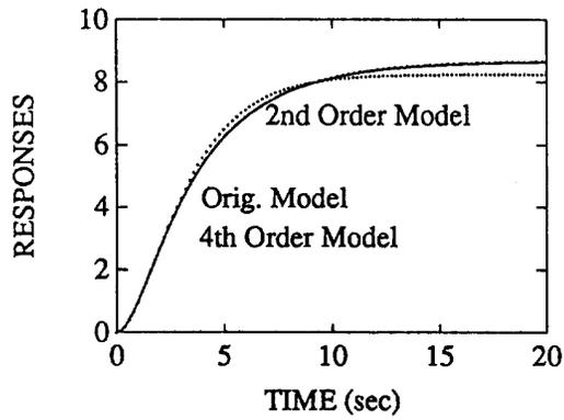
Figure 1. Step response  $y_1$  to input  $u_1$
