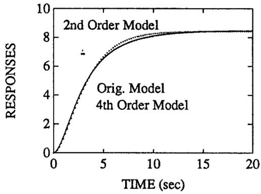
Figure 3. Step response  $y_1$  to input  $u_2$
