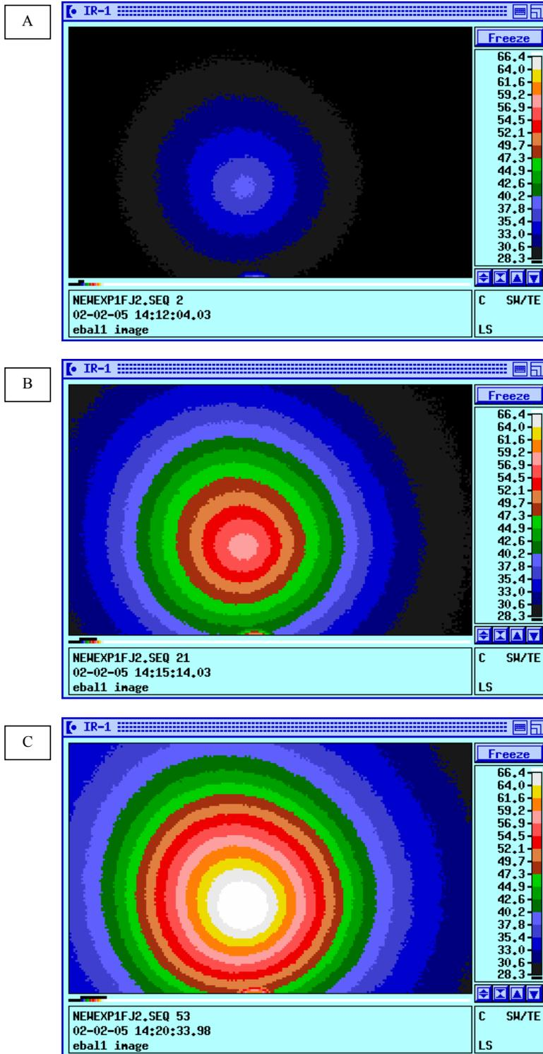
Figure 3: Flow and heat transfer visualization for single inline nozzle.
