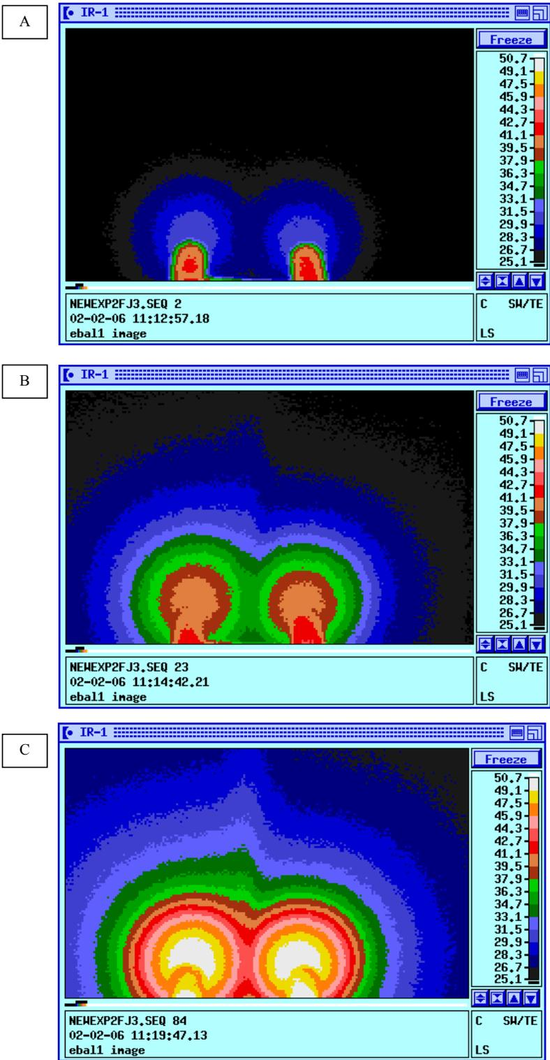
Figure 4: Flow and heat transfer visualization for Double inline nozzle.
