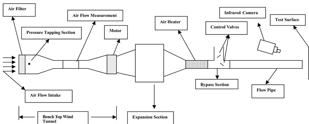
Figure 1: Heat Transfer Air Jet Impingement Experimental Facility.
