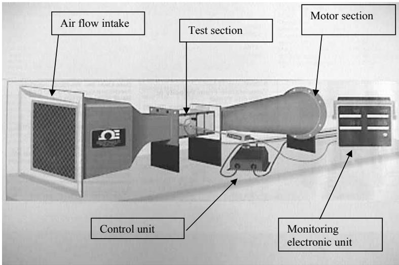
**Figure 2. Wind tunnel test and calibration facility**
