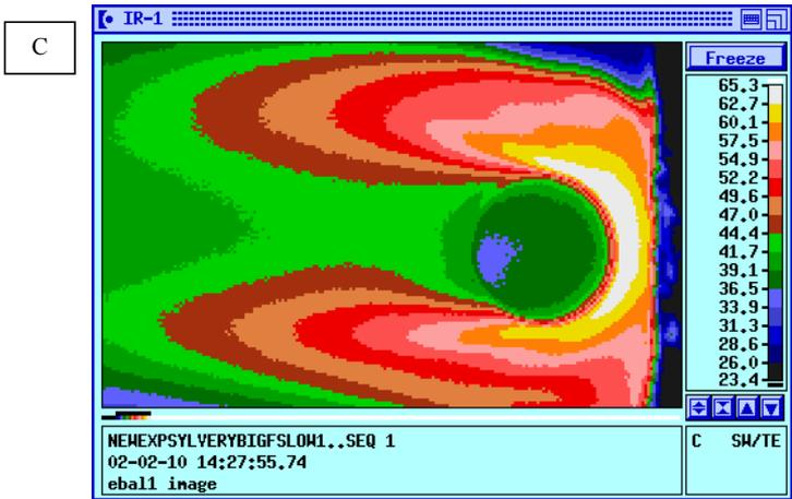
Figure 6: Flow and heat transfer visualization around a cylinder.
