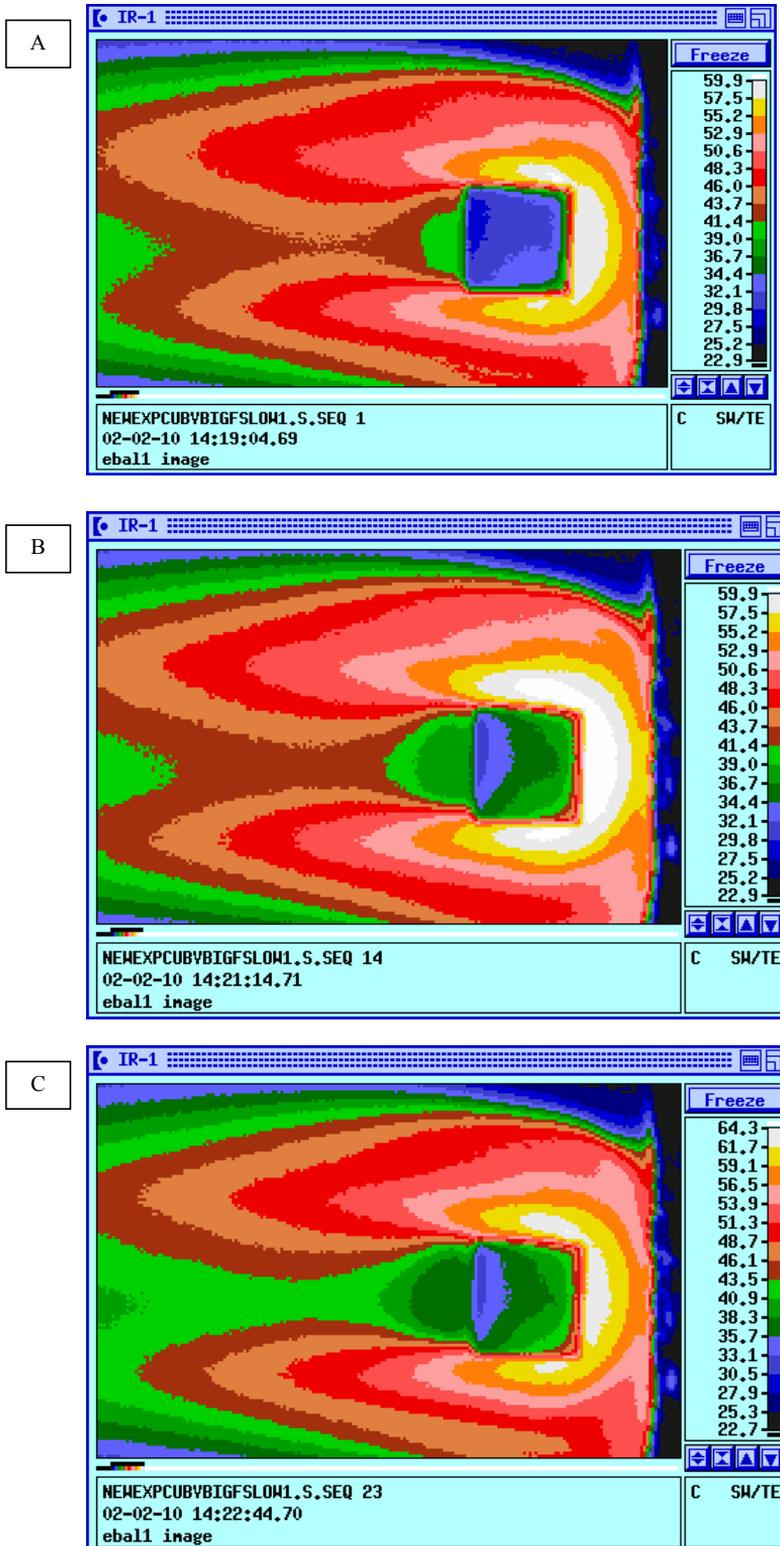
Figure 5: Flow and heat transfer visualization around a cube.
