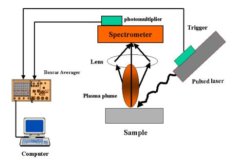
Figure:1 Schematics of the experimental setup for the geological rock analysis
