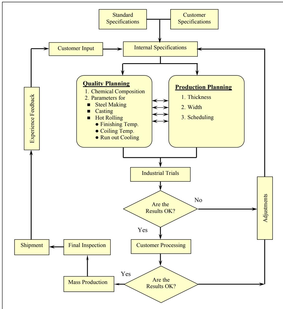
Figure 2. Product Development Loop used at Hadeed for API Steel Grades.
