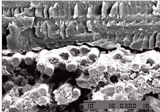
**Fig. 9** SEM fractograph showing matrix cracking and warp fiber splitting and bundle fiber fracture.
