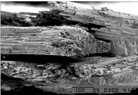
**Fig. 10** SEM fractograph showing fiber bundle fracture and delamination in class 2 laminate.
