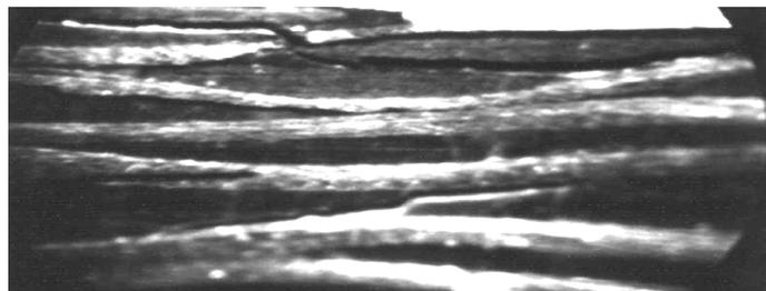
**Fig 5 (b)** Photomicrograph showing matrix cracks and delamination at 70% of fatigue life for the laminate shown in 5(a). 40x
