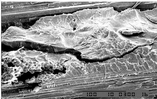
**Fig. 12** SEM Micrograph showing matrix cracking at 100°C in a Class 1 [0]<sub>8</sub> laminate.
