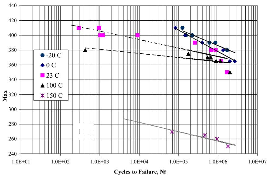
Fig. 1 Fatigue test results (SN curves) for class 1  $[0]_8$  laminates at various test temperatures
