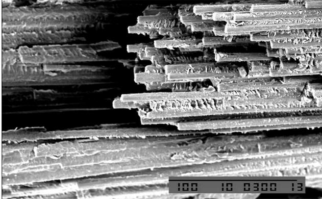
**Fig. 13** SEM fractograph showing the effect of temperature on fiber/matrix bonding at 24°C in a Class 1 laminate.
