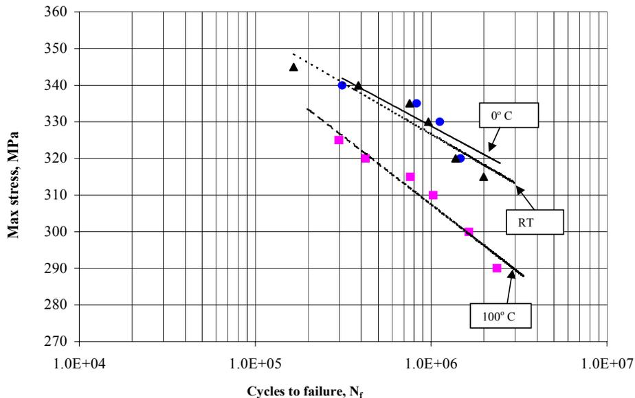
Fig. 2 Fatigue test results (SN curves) for class 2  $[0,0,45,-45]_s$  laminates at various test Temperatures.
