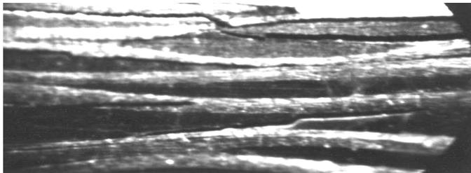
**Fig. 5 (a)** Photomicrograph showing matrix cracks and delamination at 50% of fatigue life for a class 1 laminate. 40x
