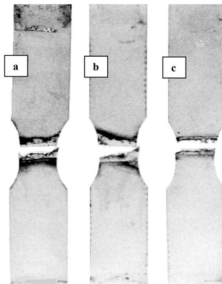
**Fig. 7** X-ray radiograph showing delamination in class 2 laminate at (a) 100°C, (b) RT (c) 0°C.
