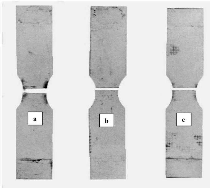
**Fig. 6** X-ray radiograph showing failure at (a) room temperature, (b) -20°C and (c) 0°C for Class 1 laminates.
