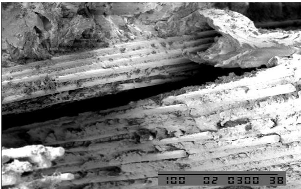
**Fig. 15** SEM fractograph showing the disintegration of matrix at 150°C in class 1 laminate.
