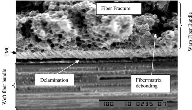
**Fig. 8** SEM fractograph showing damage events in a Class 1 [0]<sub>8</sub> laminate.
