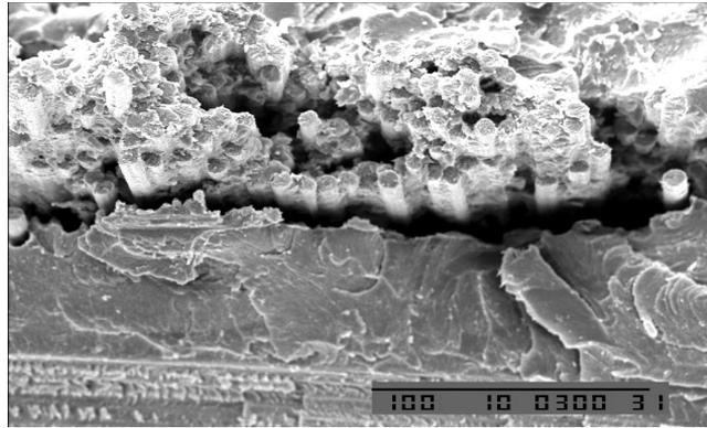
**Fig. 14** SEM fractograph showing the effect of temperature on fiber/matrix bonding at 100°C in a Class 1 laminate.
