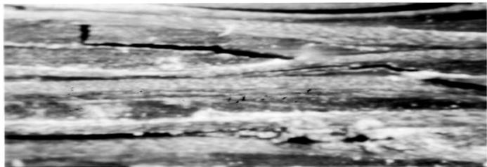
**Fig. 4** Photomicrograph showing matrix crack and delamination in a Class 1[0]<sub>8</sub> laminate. 40x
