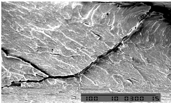
**Fig. 11** SEM fractograph showing matrix cracking at Room temperature in a Class 1 [0]<sub>8</sub> laminate.
