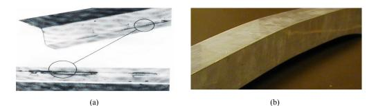
**Figure-9** Stains/oil patches (a) show as a yellow to brown area of surface discoloration, while twists and bends (b) occur due to a winding departure from straightness.
