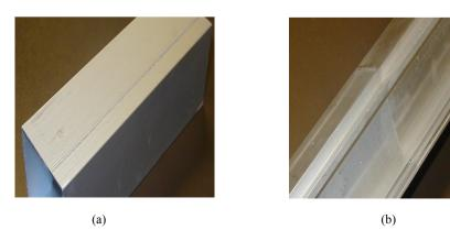
**Figure-5** A die line (a) is a longitudinal depression or protrusion formed on the extruded surface, while a weld line (b) may be due to an imperfect billet-to-billet joint.
