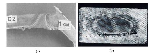
Figure-3 Pipe or extrusion defect, also known as back-end condition [Sheppard, 1999].
