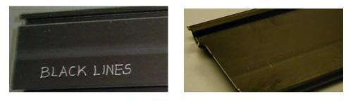
Figure-7 Black lines show as burnt surfaces on the extrudate due to local high pressures/temperatures.
