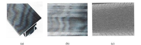
**Figure-6** Surface appearance due to die design or bearing streaking (a), ingot (billet) structure streaking (b), and surface cracking / tearing (c) [Aluminum Association 1993, Sheppard 1999].
