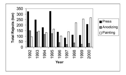
Figure 12 Comparison of rejects at the three cost centers over a 10-year period.
