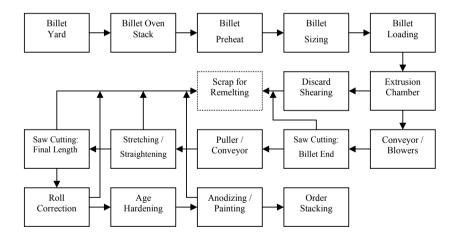
Figure-1 Process flow in commercial hot extrusion of Al-6063 [Arif et al., 2001]
