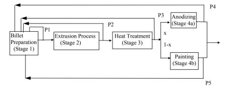
Figure-14 Plant layout showing cost centers and fraction of defectives at each stage
