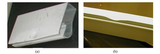
Figure-10 Damages (a) and dents (b) are categories of handling and traffic defects.
