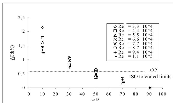
Figure 4 – Discharge Coefficient Shift for the Orifice Flow meter ( $\beta=0.7$ ) placed at Different Locations Downstream of a 90° Double Bend out of planes
