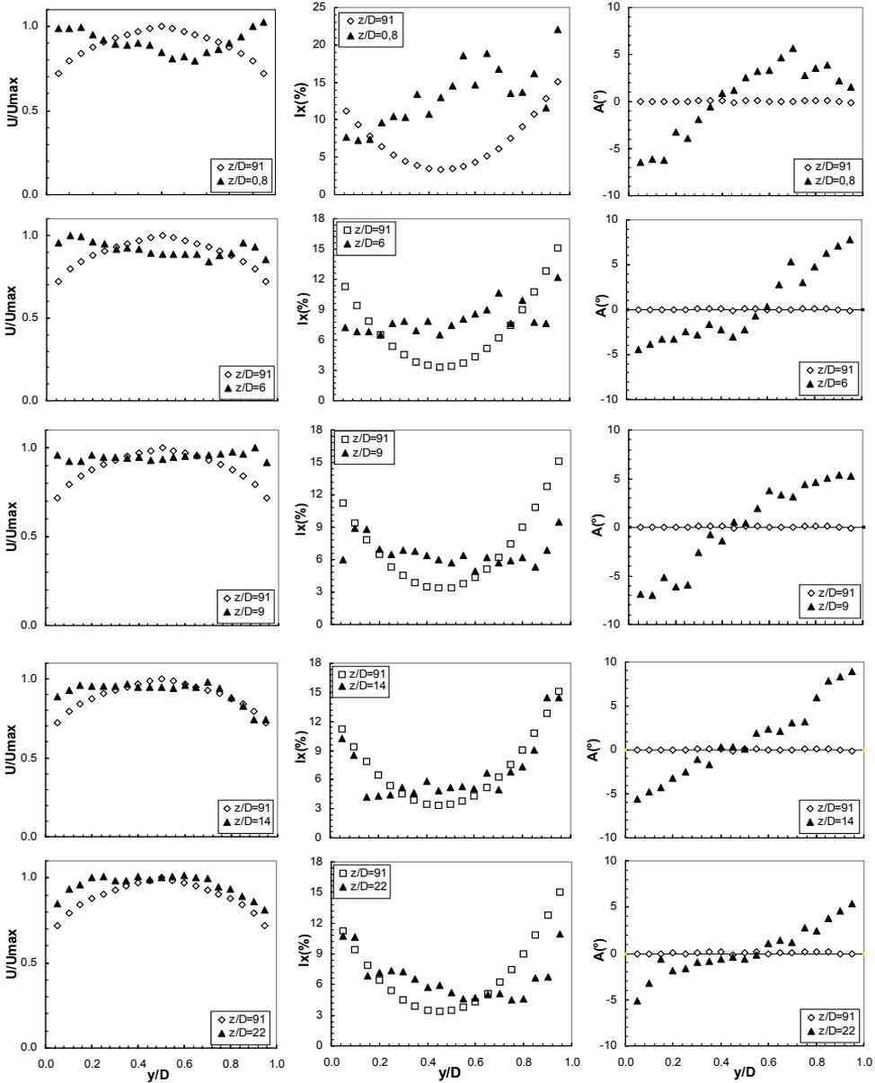
Figure 3 – Distribution of axial mean velocity, turbulence intensity and swirl angle downstream of the double bend out of plane
