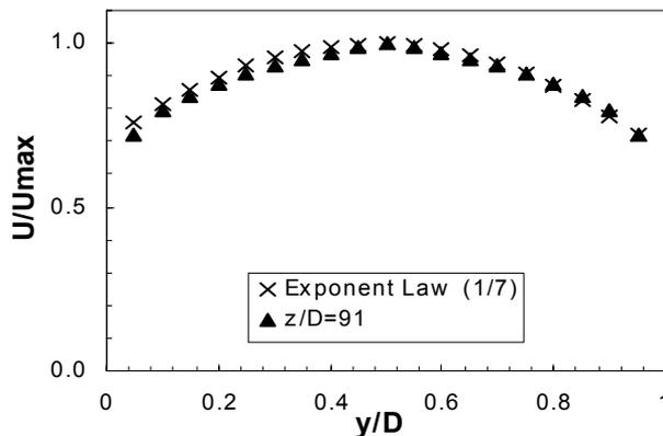
Figure 2 – Comparison of the LDA axial profile measured at 91 D downstream of the double bend with the  $(1/7)^{\text{th}}$  power law profile
