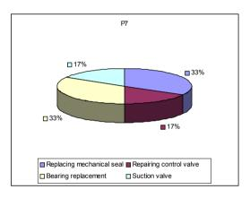
Figure 1. Modes of failure of most critical bad actor pump P7.
