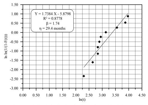
Figure 7. Weibull analysis of bearings for all typesof most critical bad actors pumps.
