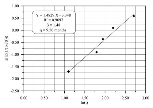
Figure 5. Weibull plot for most critical bad actor pump P7.
