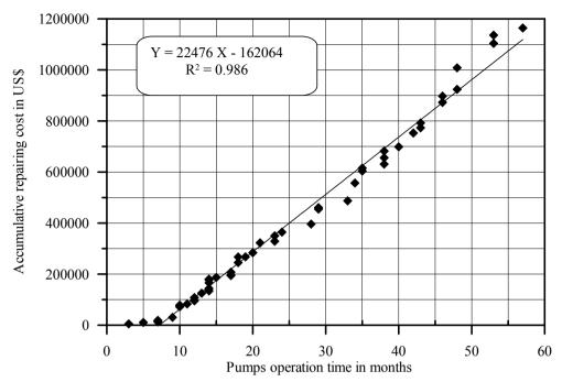
Figure 10. Accumulative repairing cost for seals of all pumps versus operation time.
