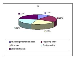
Figure 2. Modes of failure of most critical bad actor pump P3.
