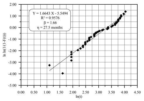
Figure 6. Weibull analysis of seals for all types of most critical bad actors pumps.
