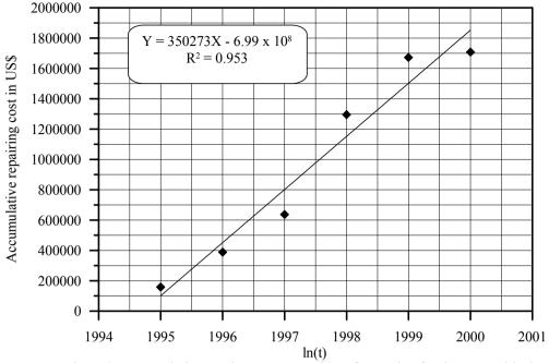
Figure 8. Accumulative repair costs versus time of operation for the most critical bad actors pumps (all failure modes).
