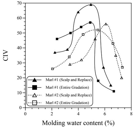
Figure 11. The CIV-moisture relationships for both marls using the large mold
