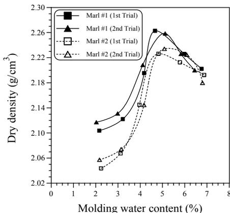
Figure 4. The moisture-density relationships for both marls using two trials
