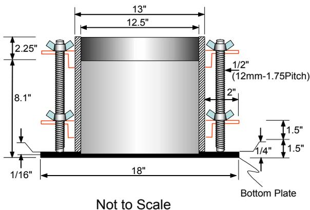
Figure 3. The large-size mold and accessories
