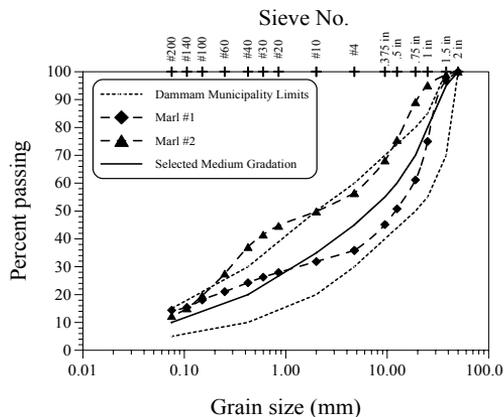
Figure 2. Grain size distribution of the collected materials and the selected gradation for the testing program
