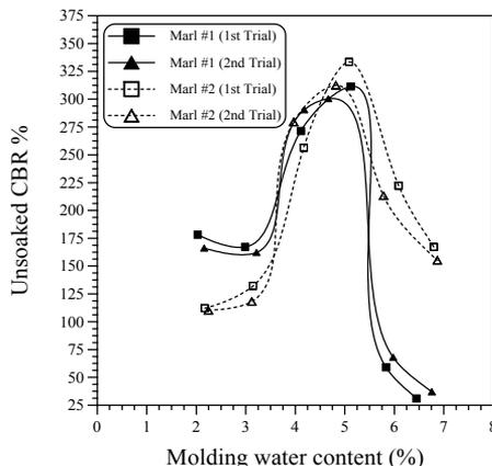
Figure 5. The CBR-moisture relationships for both marls using two trials
