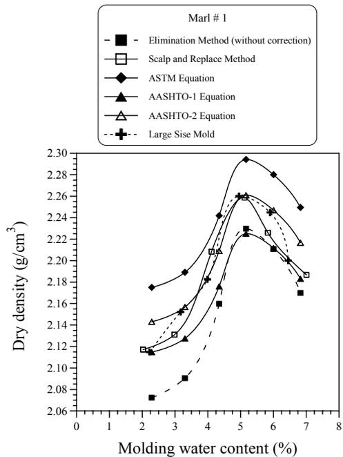
Figure 12. The moisture-density relationships for Marl #1 using different correction methods
