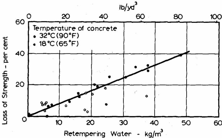
Figure 1: Effect of retempering on the compressive strength of concrete. (Neville, 1995)
